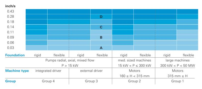
**DIN ISO 10816:** Mechanical vibrations – assessment of the vibrations of machine through measurements on no rotating parts. **Vibration velocity (rms)** 10 - 1000 Hz,  $n > 600 \text{ min}^{-1}$ , 2 - 1000 Hz,  $n > 120 \text{ min}^{-1}$
